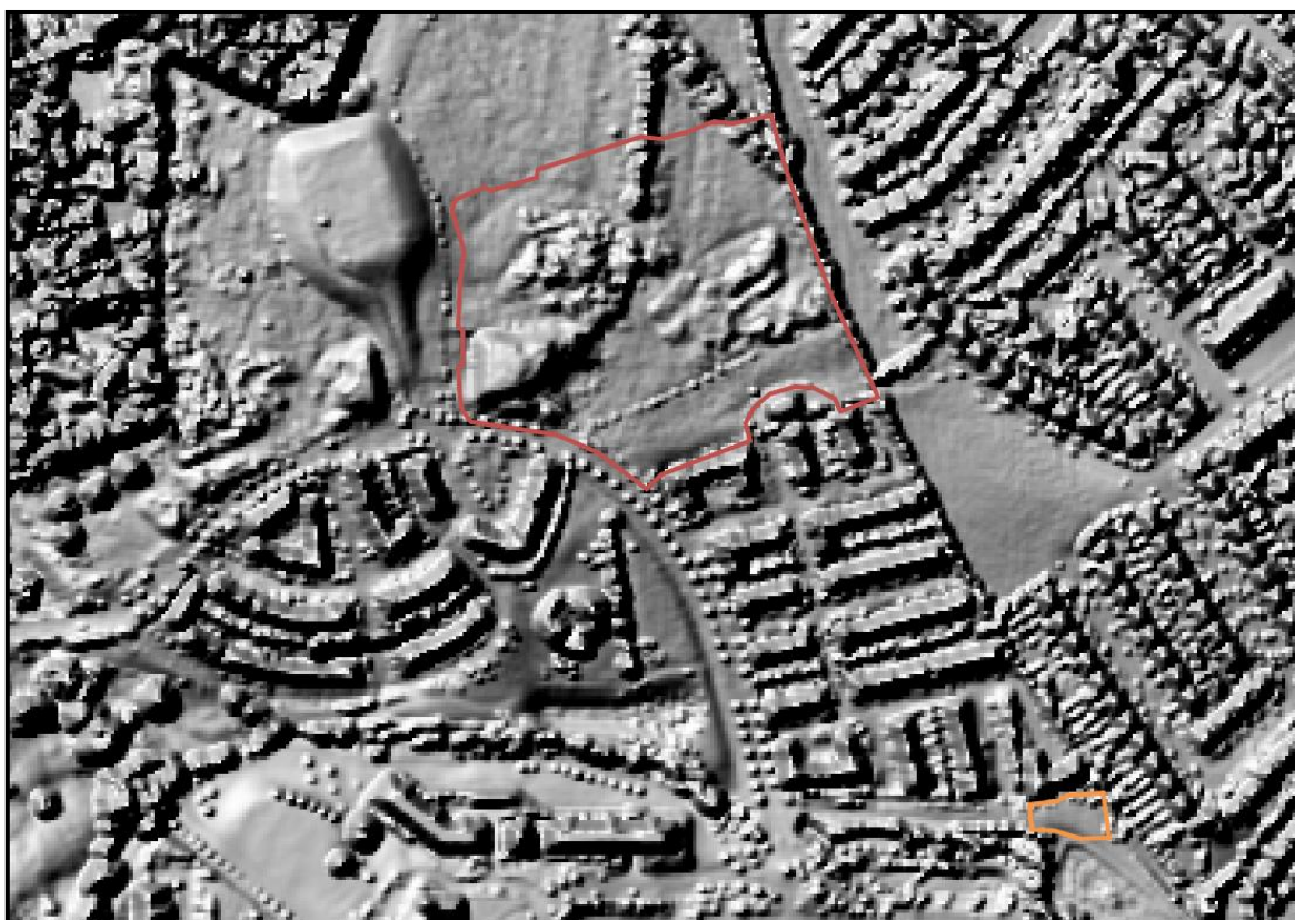
Figure 16 Extract from LiDAR image showing the proposed SHD site (in red) and proposed attenuation tank site (in orange) (Source: data.gov.ie/dataset/open-topographic-lidar-data ).
